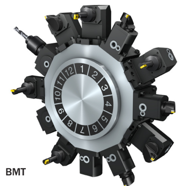
Conversion of a standard turret to Coromant Capto system
